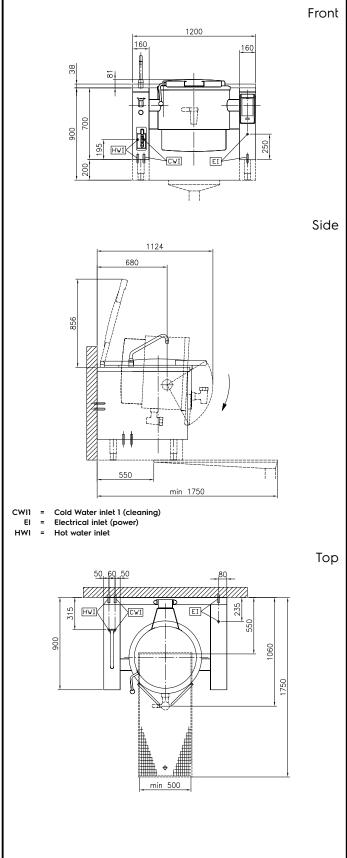
ProThermetic Sprint Electric Tilting Boiling Pan, 100lt Hygienic Profile, Freestanding with Stirrer The company reserves the right to make modifications to the products without prior notice. All information correct at time of printing.
